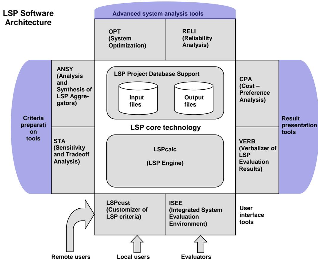
Figure 1. Component and structure of the LSP software technology
